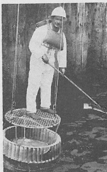
OIL SKIMMER —The Naval Air Station, Bermuda, developed this device to remove oil slicks from water near shores or around piers. Called a "platform skimmer," it uses a man, as shown, to guide the oil into the skimmer with a long-handled scraper. Once drawn into the skimmer, the oil is sucked through a hose into a tank truck on the shore or into floating fuel barge tanks or similar vessels. The device is one of several new ideas developed by the Navy to clean up pollution near port areas.
