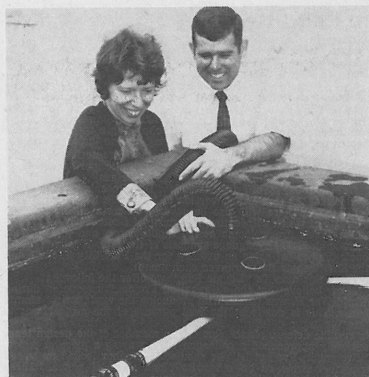
"OIL VACUUM CLEANER" —An inexpensive plastic oil removal device is tested in water and oil tanks at the Naval Civil Engineering Laboratory, Port Hueneme, Calif. In initial tests in San Diego Harbor, the "oil vacuum cleaner" picked up the same quantity of oil in five hours that would require five days to recover using currently available techniques. The device is undergoing further testing before being put out into Navy-wide use and being made available for civilian application.
